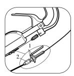
Unscrew the lock nuts (1) and screw the adjuster (2) in or out as necessary. Tighten the locknuts (1) when correctly adjusted.
